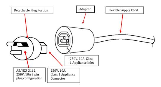
Note: the adaptor part fits within scope of AS/NZS 60320.2.2 as a plug connector
